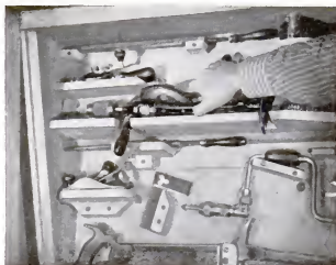
Cabinet shelves tilt backwards slightly and are designed to suit the tools. Bulkier tools are stored at top. Note rabbit for plywood cover
